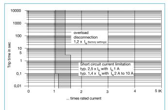
• Without the current limitation there would be a much higher overcurrent in the event of an overload or short circuit.
